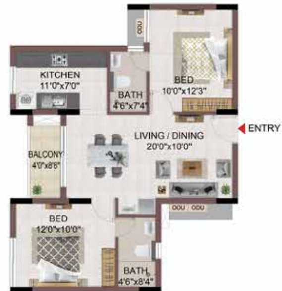
TYPICAL FLOOR 1ST TO 4TH
